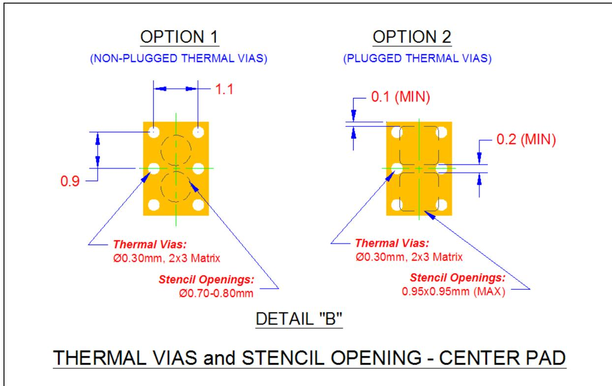
**FIGURE 6-6: CAP1296 LAND DIMENSIONS - 10-PIN DFN 3MM X 3MM**
