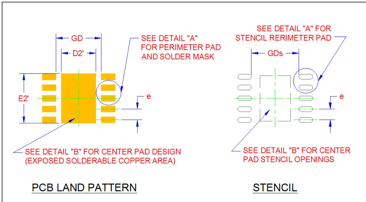
FIGURE 6-4: CAP1296 PCB DETAIL A - 10-PIN DFN 3MM X 3MM
