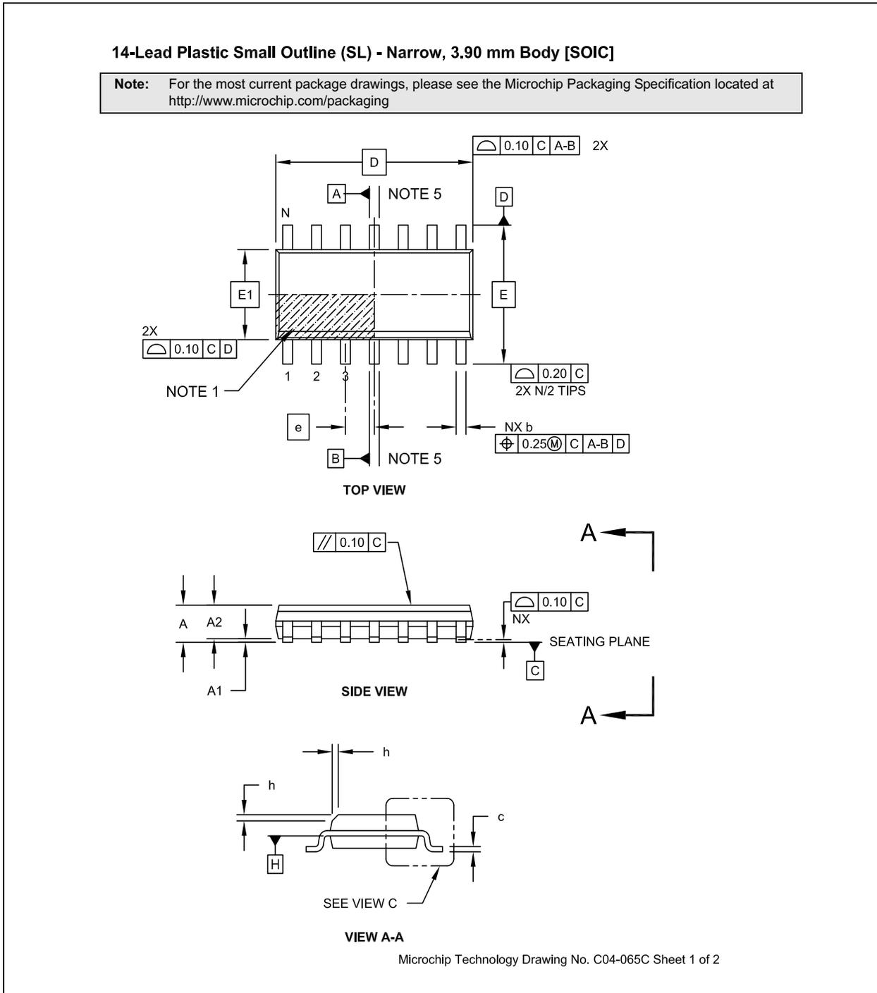
**FIGURE 6-7: CAP1296 14-LEAD PLASTIC SMALL OUTLINE, NARROW, 3.90 MM BODY (SOIC)**
