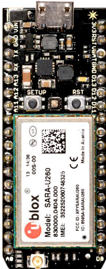
The Electron has a footprint, which is a drop-in compatible with the Particle Photon or Core.
