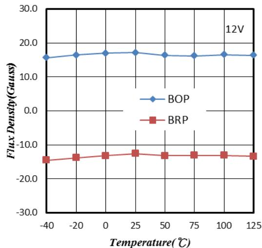
Figure 2. Flux Density vs. Temperature
