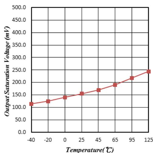
Figure 6. Saturation Voltage vs. Temperature
