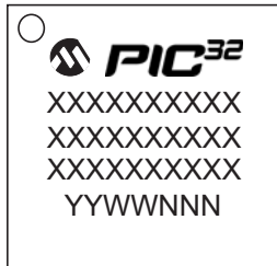
64-Lead TQFP (10x10x1 mm)
