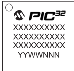
64-Lead TQFP (10x10x1 mm)
