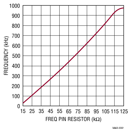
Figure 2. Switching Frequency vs Resistor on FREQ pin
