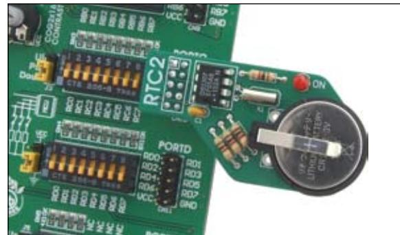
Figure 2: RTC2 placed on the development system
