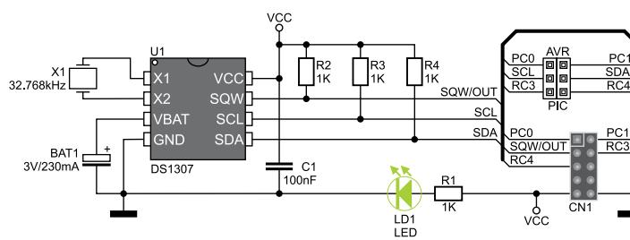
Figure 4: RTC2 connection schematic
