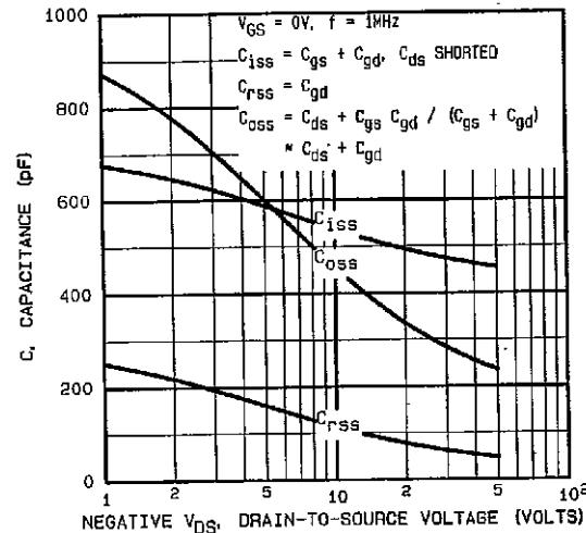
**Fig. 9 - Typical Capacitance vs. Drain-to-Source Voltage**
