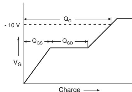
**Fig. 19 - Basic Gate Charge Waveform**
