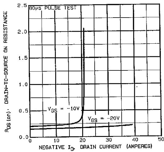
Fig. 11 - Typical On-Resistance vs. Drain Current
