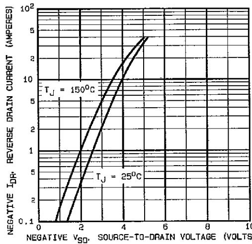
**Fig. 6 - Typical Source-Drain Diode Forward Voltage**
