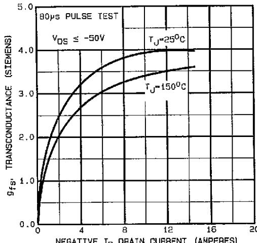
**Fig. 5 - Typical Transconductance vs. Drain Current**
