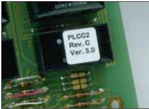
Circuit Board Labeling
