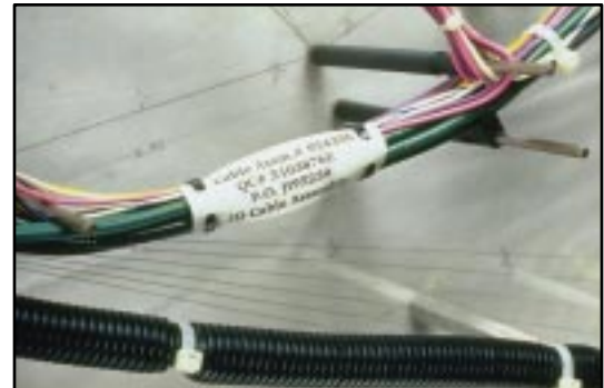
Identify harness board assemblies
