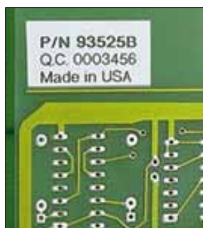
Circuit board labeling
