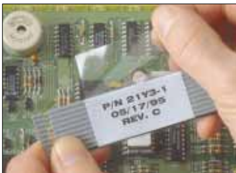
Flat Ribbon Cable Labeling
