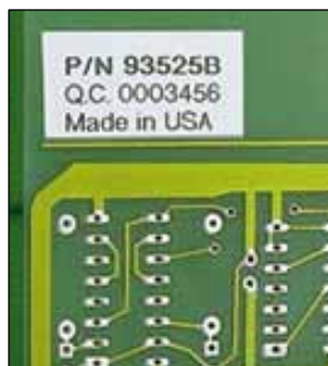
Circuit board labeling
