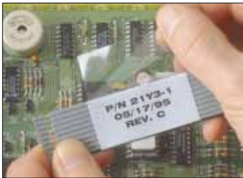
Flat Ribbon Cable Labeling
