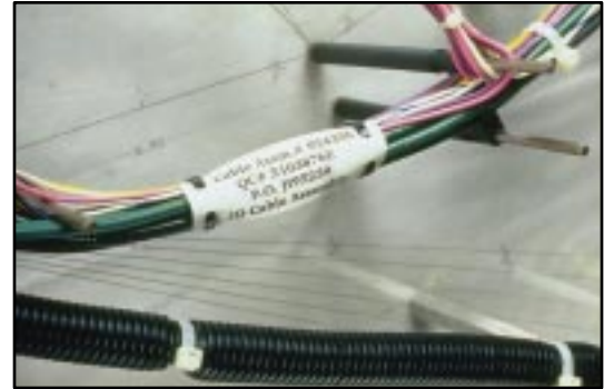
Identify harness board assemblies
