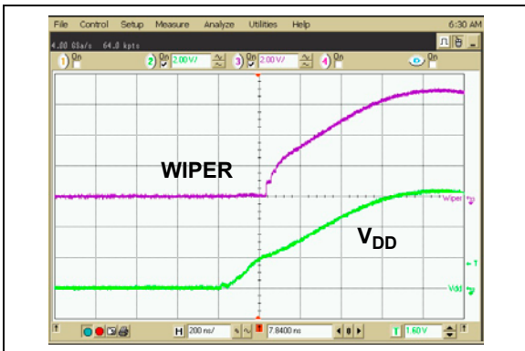
FIGURE 2-15: 2.1 k \Omega – Power-Up Wiper Response Time.
