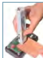
Verify the effectiveness of shielding
