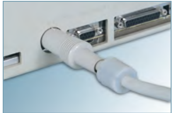
I/O cable with RFI suppressor.
