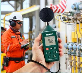
Extech's ultra-compact sound meter meets class 2 standards with  $\pm 1$ dB high accuracy that allows for quick and reliable sound level testing. It features a large backlit display for easy viewing and measures A & C weighting from 35 to 130dB with Fast and Slow response time mode. Size is small enough to conveniently fit in your pocket and includes a wrist strap.
