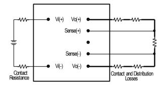
Figure 16: Effective circuit configuration for remote sense operation
