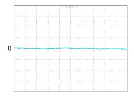
**Figure 12:** Input reflected ripple current, i<sub>s</sub>, through a 12µH source inductor at nominal input voltage and rated load current (20 mA/div, 2us/div)
