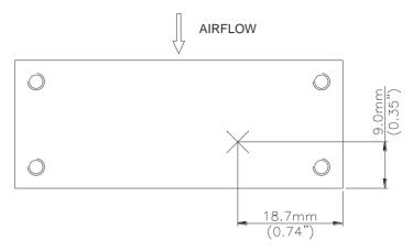
**Figure 22:** \* Hot spot 2 temperature measured point. The allowed maximum hot spot 2 temperature is defined at 105  $^\circ$ C
