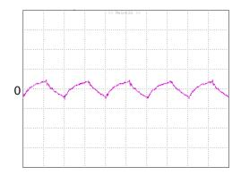
**Figure 14:** Output voltage ripple at nominal input voltage and rated load current (Io=40A)(100 mV/div, 1us/div)
