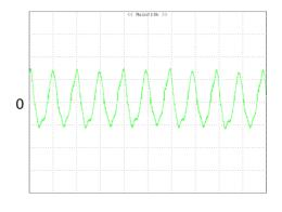
**Figure 11:** Input Terminal Ripple Current, i<sub>c</sub>, at full rated output current and nominal input voltage with 12μH source impedance and 100μF electrolytic capacitor (100 mA/div, 2us/div)
