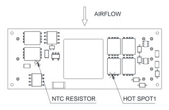
**Figure 20:** \* Hot spot 1& NTC resistor temperature measured points. The allowed maximum hot spot 1 temperature is defined at 117  $^{\circ}$
