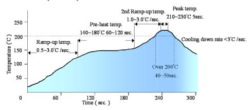
Note: The temperature refers to the pin of E48SP, measured on the pin +Vout joint.
