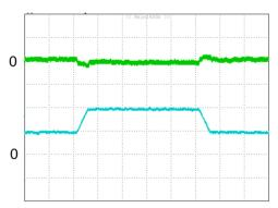
**Figure 8:** Output voltage response to step-change in load current (75%-50%-75% of Io, max; di/dt = 0.1A/ $\mu$ s). Load cap:  $10\mu$ F tantalum capacitor and  $1\mu$ F ceramic capacitor. Top Trace: Vout (100mV/div, 200us/div), Bottom Trace: lout (10A/div). Scope measurement should be made using a BNC cable (length shorter than 20 inches). Position the load between 51 mm to 76 mm (2 inches to 3 inches) from the module
