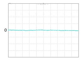
**Figure 12:** Input reflected ripple current, i<sub>s</sub>, through a 12µH source inductor at nominal input voltage and rated load current (20 mA/div, 2us/div)
