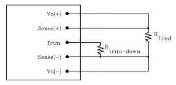
Figure 17: Circuit configuration for trim-down (decrease output voltage)
