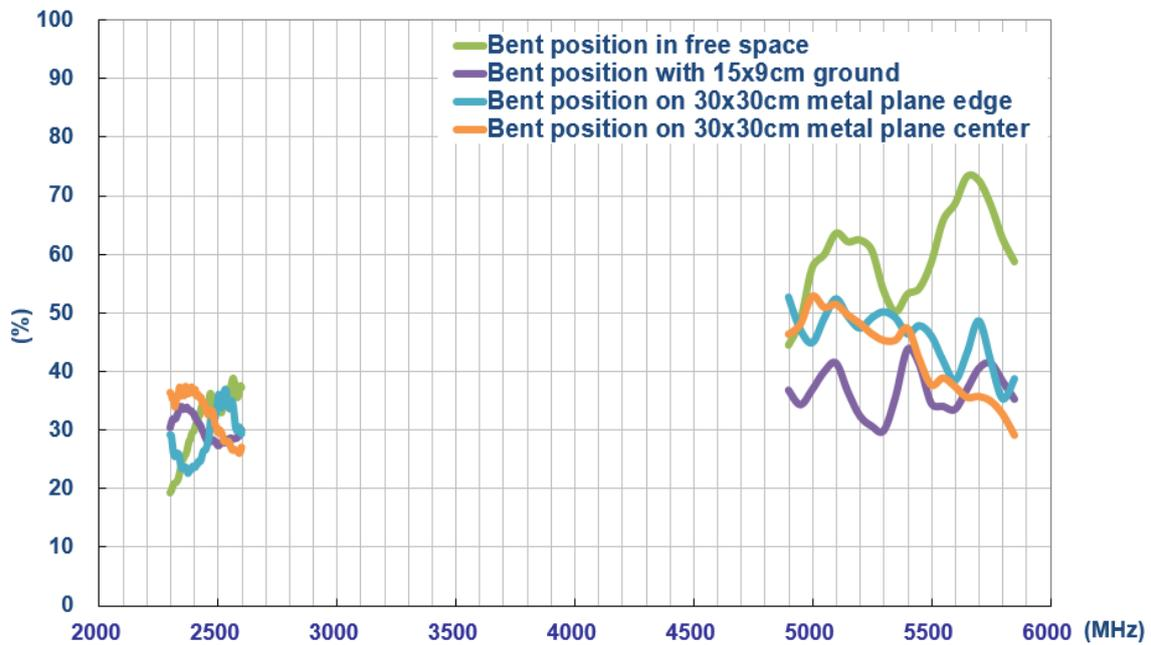
**Figure5.** Efficiency of GW.05 antenna with bent position
