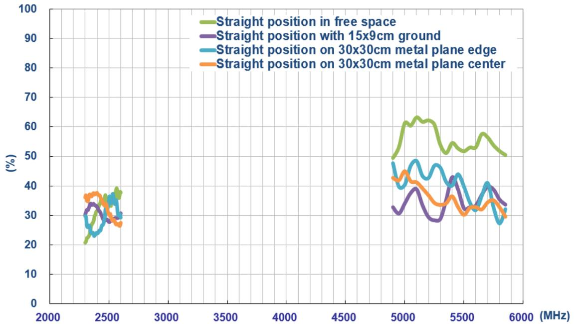
**Figure4.** Efficiency of GW.05 antenna with straight position
