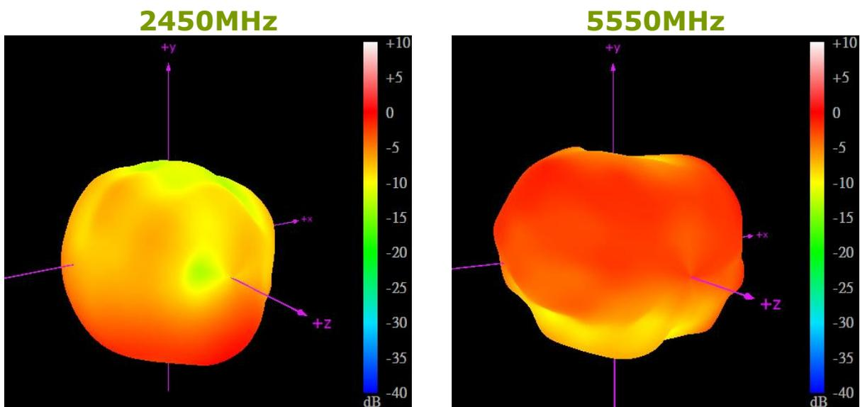
**4.11 3D Radiation Pattern (Straight position with 30x30cm ground plane edge)**
