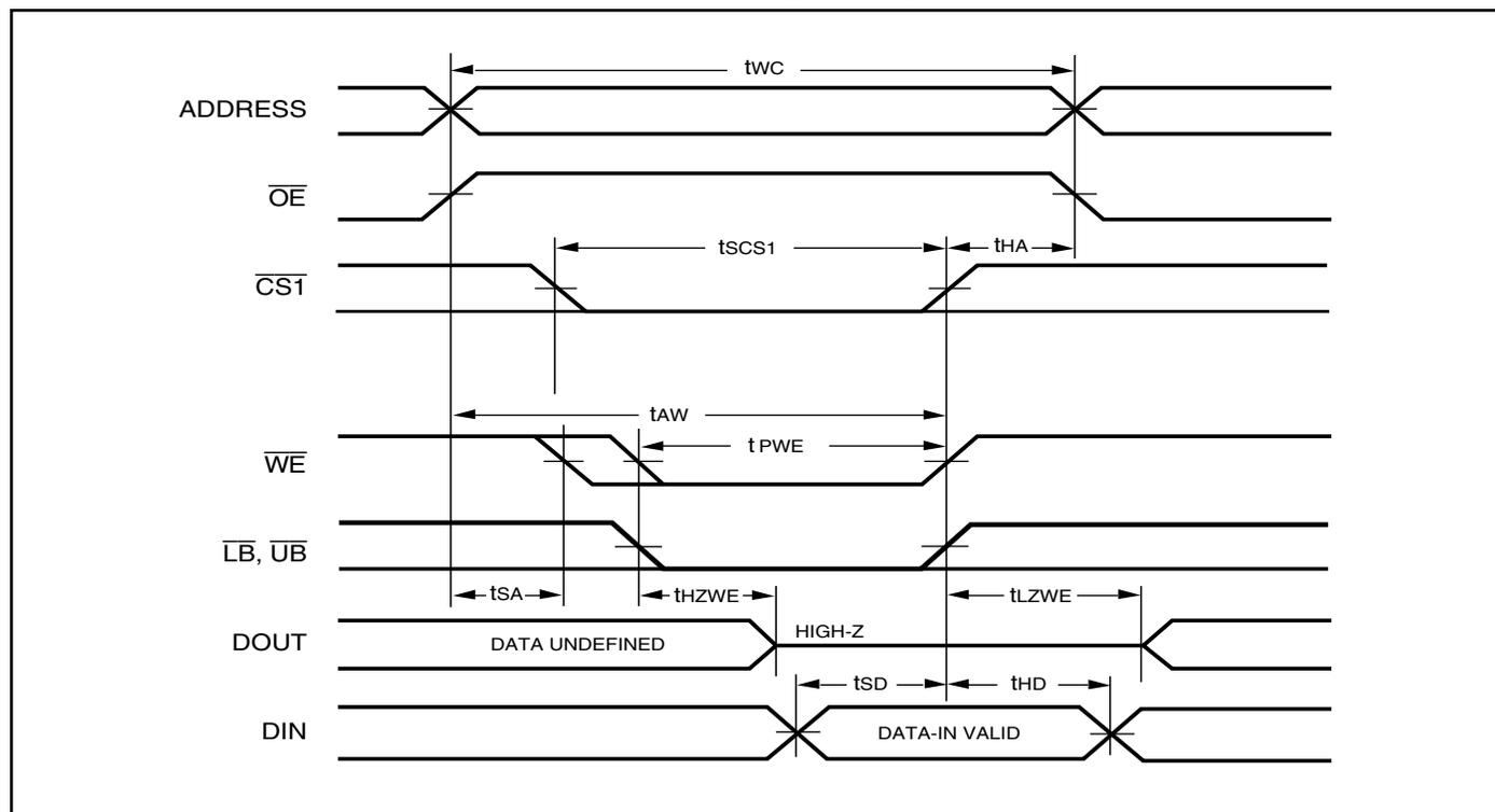
**WRITE CYCLE NO. 3** ( $\overline{WE}$  Controlled:  $\overline{OE}$  is LOW During Write Cycle)
