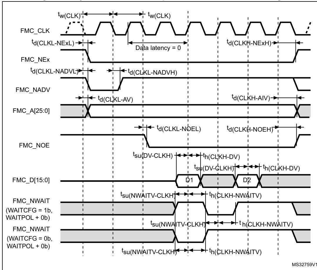
Table 107. Synchronous non-multiplexed NOR/PSRAM read timings<sup>(1)(2)(3)</sup>
