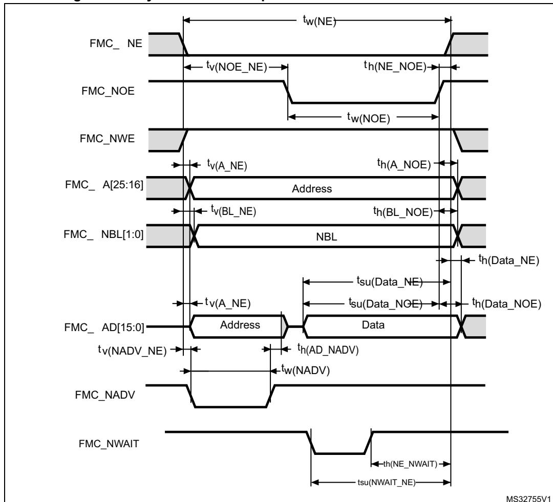
**Table 101. Asynchronous multiplexed PSRAM/NOR read timings<sup>(1)(2)</sup>**
