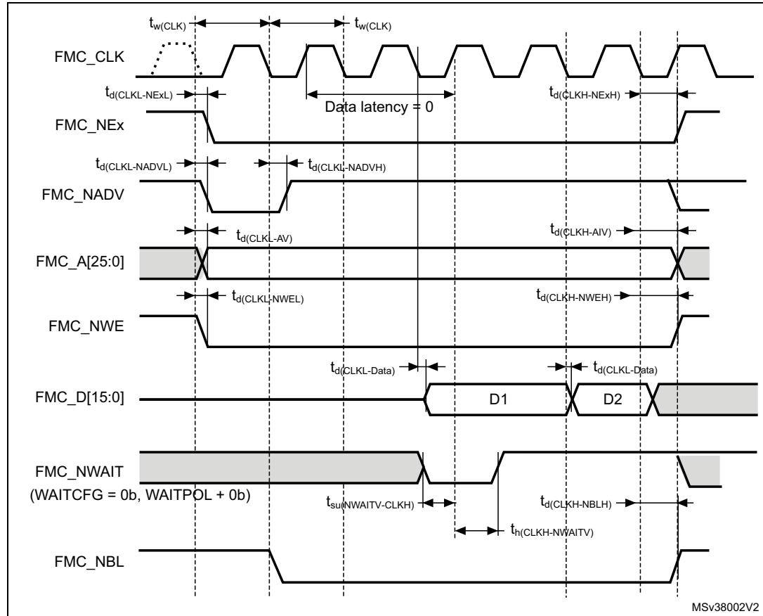
**Table 108. Synchronous non-multiplexed PSRAM write timings<sup>(1)(2)(3)</sup>**
