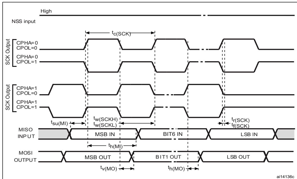
1. Measurement points are done at CMOS levels: 0.3 V<sub>DD</sub> and 0.7 V<sub>DD</sub>.
