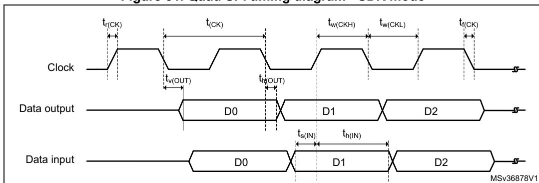
**Figure 52. Quad SPI timing diagram - DDR mode**
