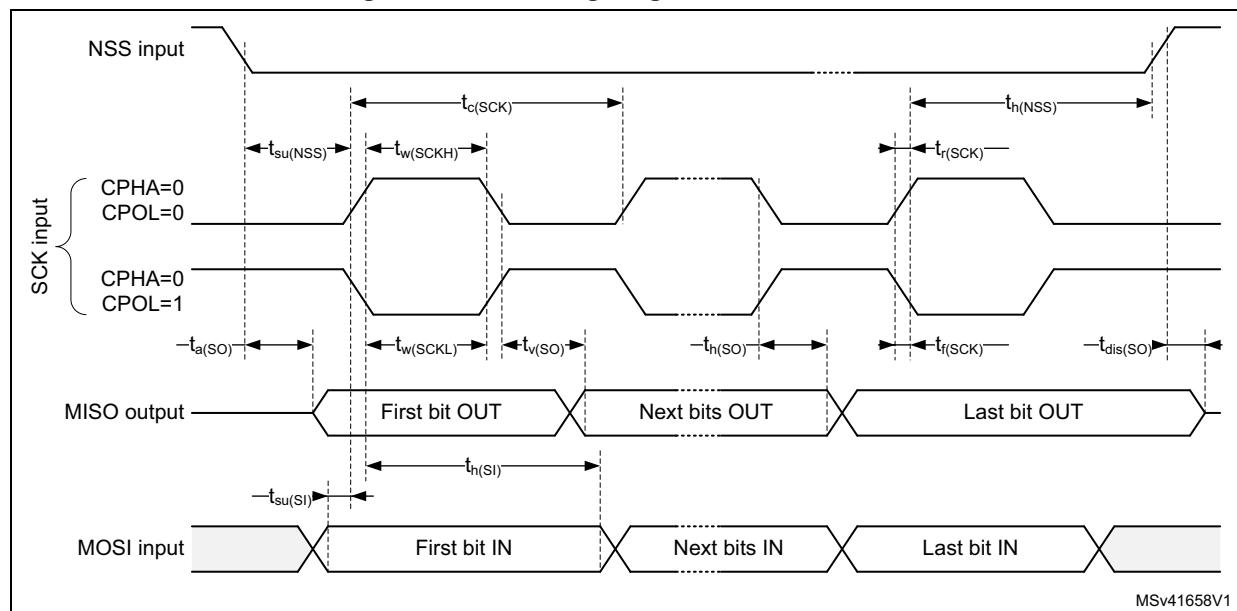
Figure 35. SPI timing diagram - slave mode and CPHA = 1
