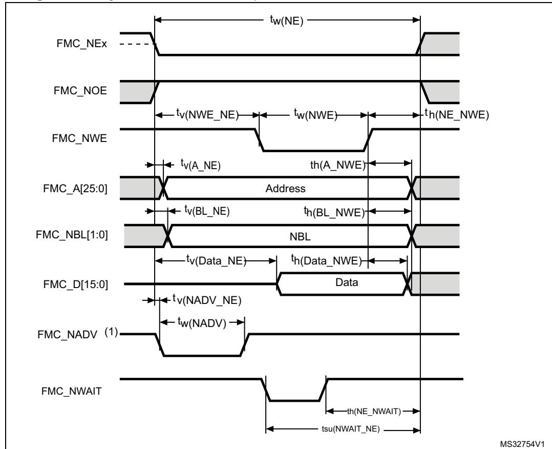
**Table 99. Asynchronous non-multiplexed SRAM/PSRAM/NOR write timings<sup>(1)(2)</sup>**
