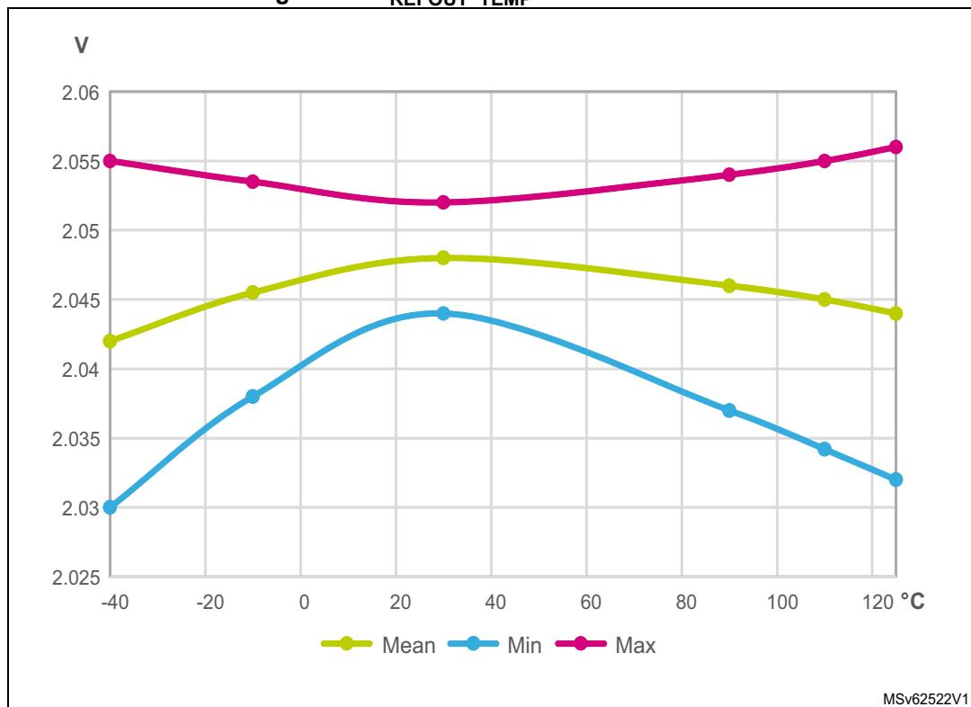
**Figure 31.  $V_{REFOUT\_TEMP}$  in case VRS = 01**
