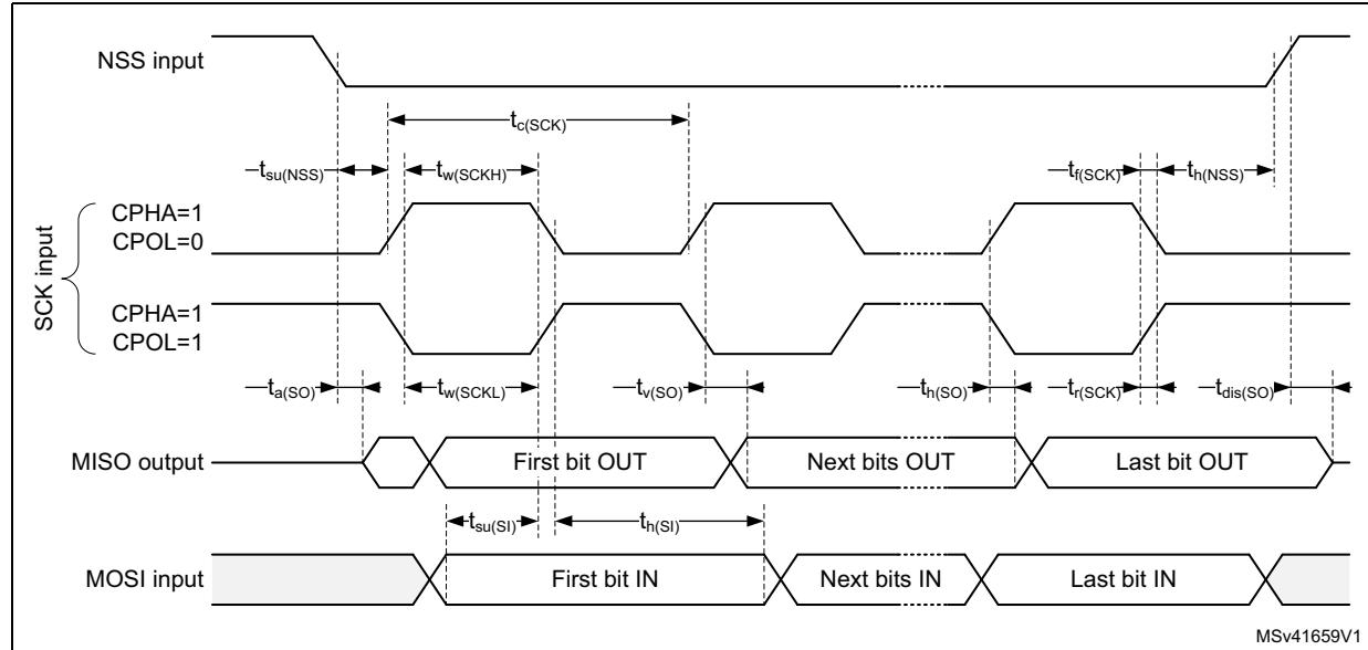
1. Measurement points are done at CMOS levels: 0.3 V<sub>DD</sub> and 0.7 V<sub>DD</sub>.
