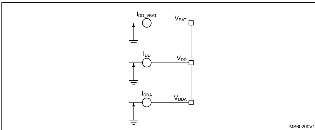
The  $I_{DD\_ALL}$  parameters given in [Table 21](#) to [Table 28](#) represent the total MCU consumption including the current supplying  $V_{DD}$ ,  $V_{DDA}$  and  $V_{BAT}$ .
