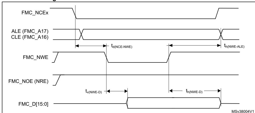
**Figure 49. NAND controller waveforms for common memory read access**
