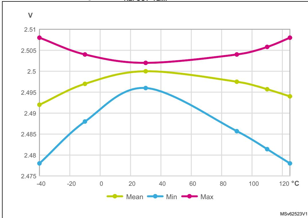
**Figure 32.  $V_{REFOUT\_TEMP}$  in case VRS = 10**
