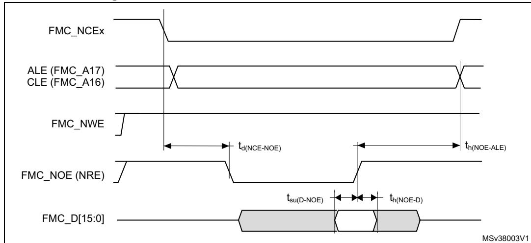
**Figure 48. NAND controller waveforms for write access**
