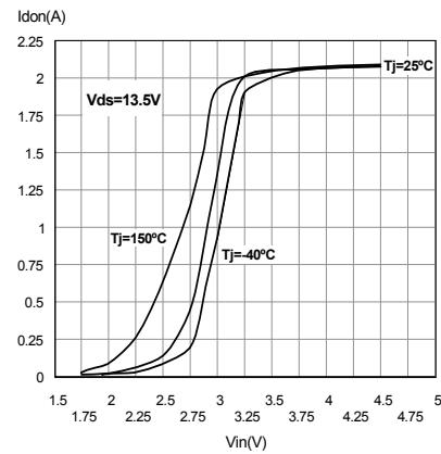
**Figure 18. Turn-on current slope (part 2/2)**
