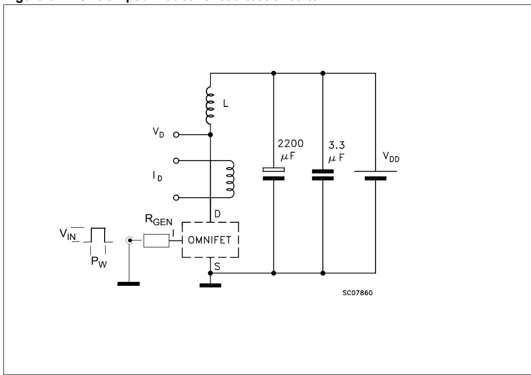
**Figure 7.** Input charge test circuit
