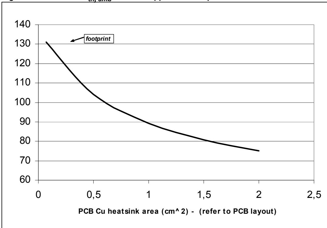
Figure 32. SOT-223 thermal impedance junction ambient single pulse
