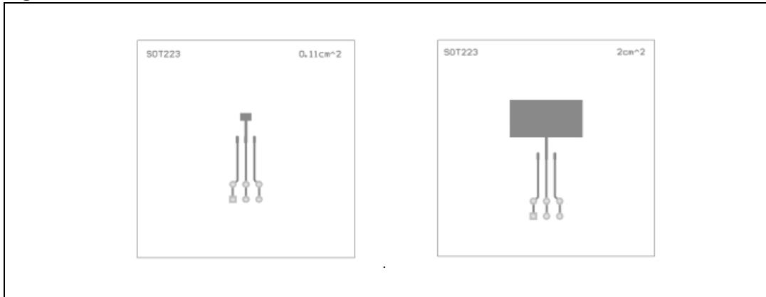
Note: Layout condition of  $R_{th}$  and  $Z_{th}$  measurements (PCB FR4 area = 58 mm x 58 mm, PCB thickness = 2 mm, Cu thickness=35  $\mu$ m, Copper areas: from minimum pad layout to 0.8 cm<sup>2</sup>).
