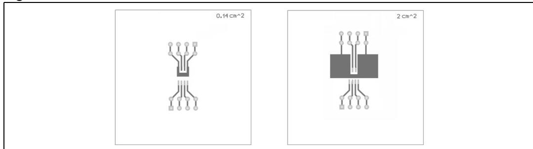
Note: Layout condition of  $R_{th}$  and  $Z_{th}$  measurements (PCB FR4 area = 58 mm x 58 mm, PCB thickness = 2 mm, Cu thickness=35  $\mu\text{m}$ , Copper areas: from minimum pad layout to 2  $\text{cm}^2$ ).
