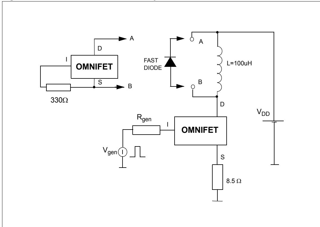
**Figure 6.** Unclamped inductive load test circuits
