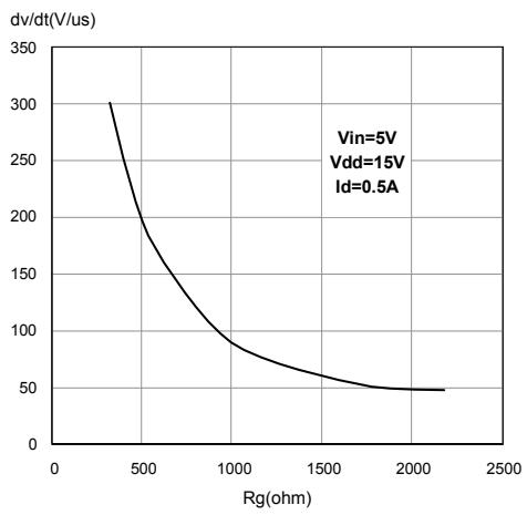
**Figure 21. Turn-off drain-source voltage slope (part 2/2)**
