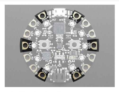
There are 6 power pads available, equally spaced around the perimeter.
