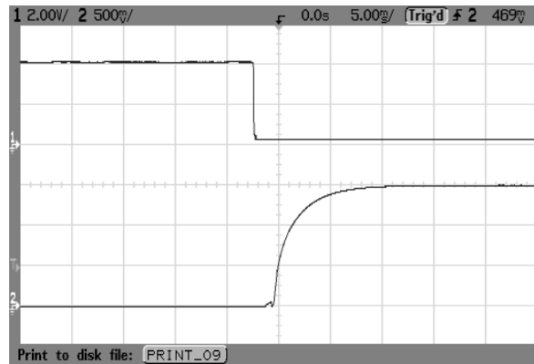
Fig.60 AVO50-48S1V5 typical start-up from CNT on
