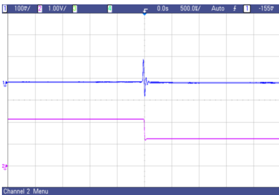
Fig.32 AVO50-48S1V8 typical transient response to step decrease in load from 50% to 25% of full load, room temperature, 48Vdc input ( \Delta I_o/\Delta t = 1A/1\mu s )
