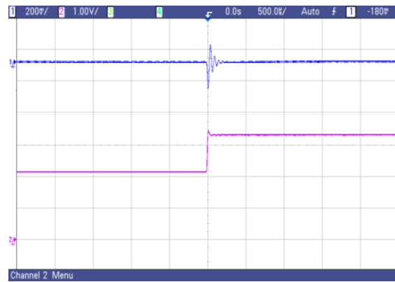
Fig.25 AVO50-48S1V5 typical transient response to step increase in load from 50% to 75% of full load, room temperature, 48Vdc input ( \Delta I_o/\Delta t = 1A/1\mu s )
