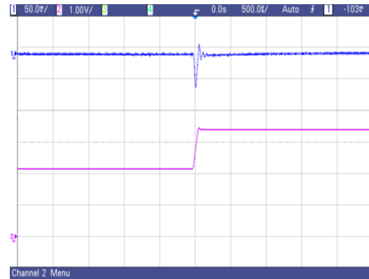
fig.23 AVO50-48s1V2 typical transient response to step increase in load from 50% to 75% of full load, room temperature, 48Vdc input ( \Delta I_o/\Delta t = 0.1A/1\mu s )
