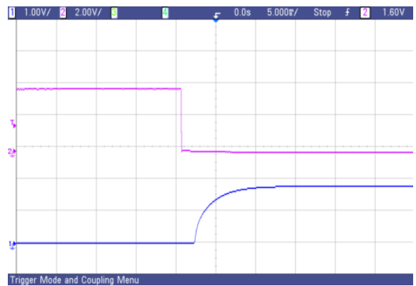
Fig.62 AVO50-48S1V8 typical start-up from CNT on
