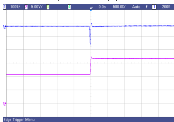
Fig.45 AVO50-48S05 typical transient response to step increase in load from 50% to 75% of full load, room temperature, 48Vdc input ( \Delta I_o/\Delta t = 1A/1\mu s )
