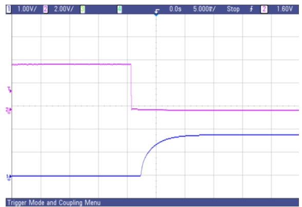
Fig.62 AVO50-48S1V8 typical start-up from CNT on
