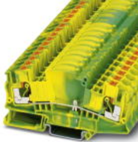
Ground modular terminal block, Connection method: Push-in connection, Cross section: 0.5 mm 2 -10 mm 2 , AWG: 20 - 10, Width: 8.2 mm, Color: green-yellow
