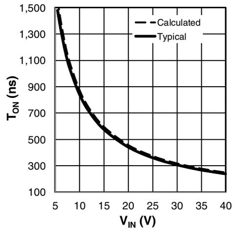
Figure 4:  $T_{ON}$  versus  $V_{IN}$ ,  $R_{ON} = 27.4k$
