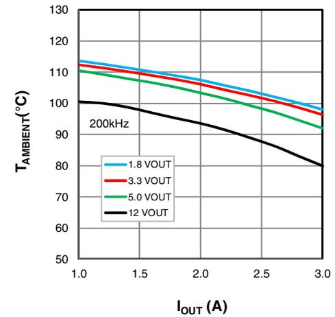
Figure 30: XR76203,  $V_{IN}=24\text{V}$
