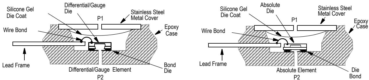
**Figure 4. Cross Sectional Diagrams (Not to Scale)**
