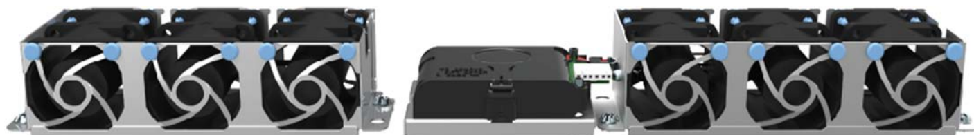
Figure 48. Support for single Intel® RAID Maintenance Free Backup Unit (Standard Option)
