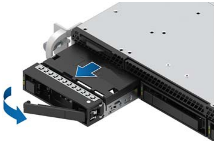
Figure 29. Drive Carrier Removal
