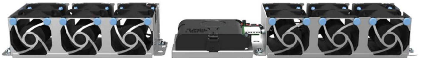
Figure 48. Support for single Intel® RAID Maintenance Free Backup Unit (Standard Option)
