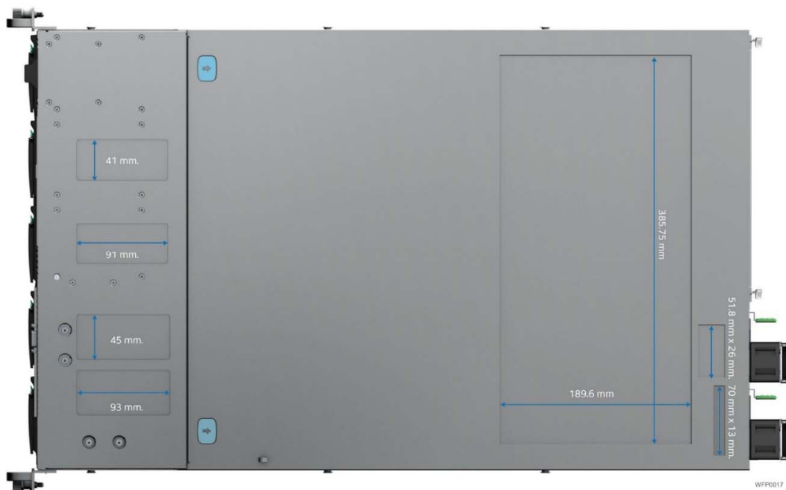
Figure 14. Label Emboss Dimensions
