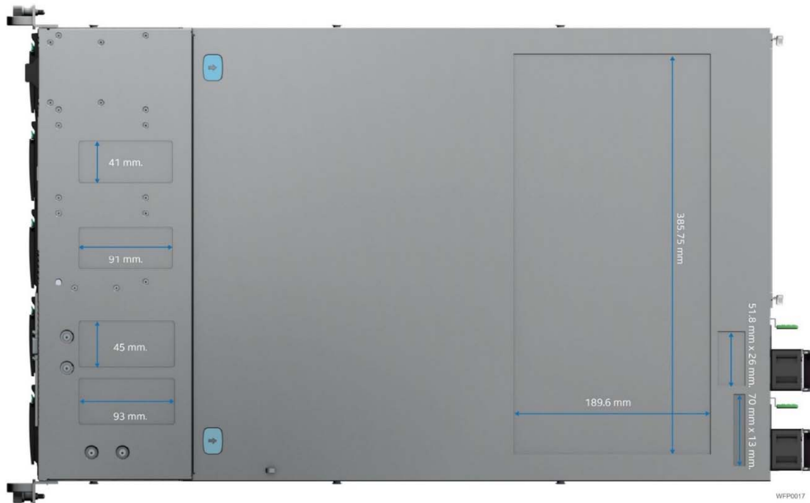
Figure 14. Label Emboss Dimensions
