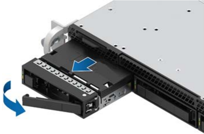
Figure 29. Drive Carrier Removal
