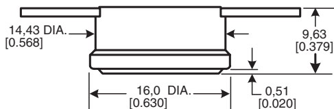
SERIES NAME 2450R Phenolic Automatic Reset Thermostat
