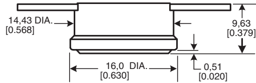
SERIES NAME 2450R Phenolic "One-shot" ½ in Thermostat
