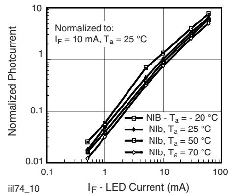
Fig. 10 - Normalized Photocurrent vs. I<sub>F</sub> and Temperature
