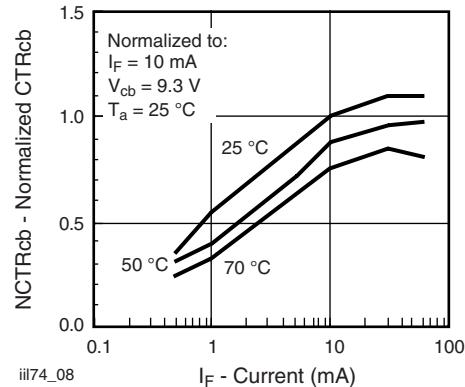
Fig. 8 - Normalized CTR<sub>cb</sub> vs. LED Current and Temperature
