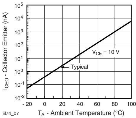
Fig. 7 - Collector Emitter Leakage Current vs. Temperature
