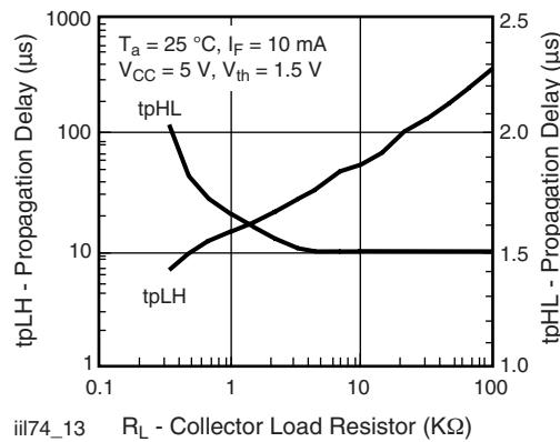
Fig. 13 - Propagation Delay vs. Collector Load Resistor
