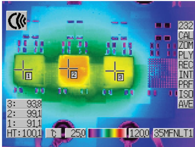
Figure 7. Thermal Capture at 12V<sub>IN</sub>, 1.0V<sub>OUT</sub> at 75A (Ambient Temperature = 23.3°C, No Airflow and No Heat Sink)
