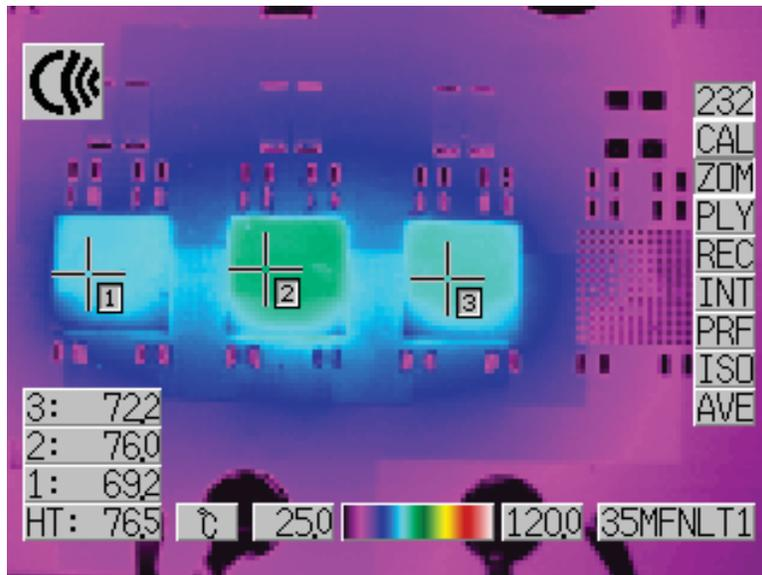
Figure 8, Thermal Capture at 12V<sub>IN</sub>, 1.0V<sub>OUT</sub> at 75A (Ambient Temperature = 23.3°C, 200LFM Airflow and No Heat Sink)
