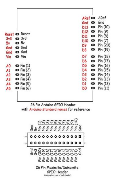
MM-BASIC allows the GPIO ports to be accessed with the PIN() command and function, and different functions to be set with SETPIN command.
