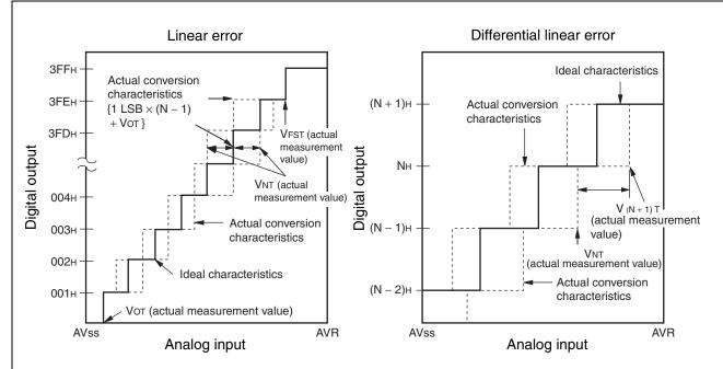
$$Linear\ error\ of\ digital\ output\ N = \frac{V_{NT} - \{1\ LSB \times\ (N-1)\ + Vor\}}{1\ LSB} [LSB]$$
