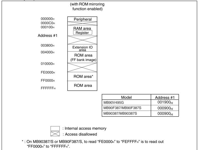
Note: When internal ROM is operating, F<sup>2</sup>MC-16LX allows viewing ROM data image on FF bank at upper-level of 00 bank. This function is called "mirroring ROM," which allows effective use of C compiler small model. F<sup>2</sup>MC-16LX assigns the same low order 16-bit address to FF bank and 00 bank, which allows referencing table in ROM without specifying "far" using pointer.
