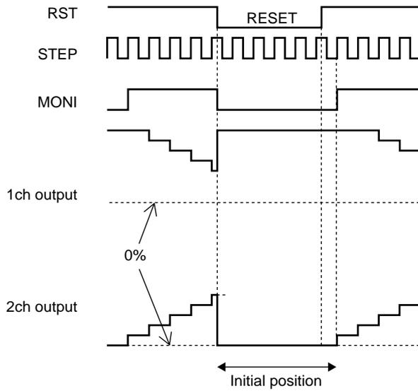
When the RST pin is set to Low, the excitation position of the output is forcibly set to the initial position, and the MONI output is placed in the ON state. When RST is then set to High, the excitation position is advanced by the next STEP input.
