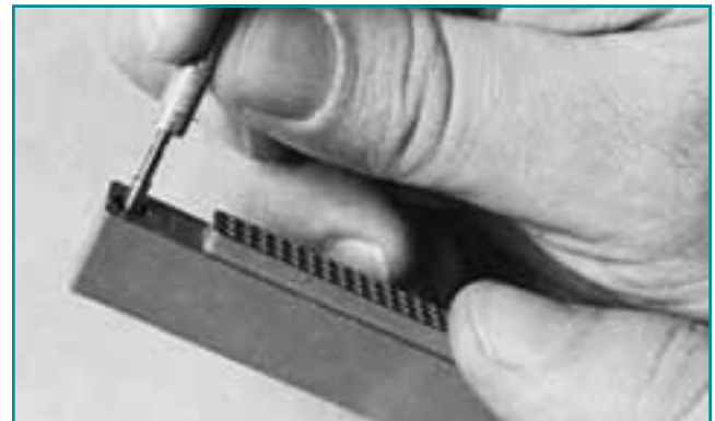
LOCKING SCREW ACCESSORY INSERTED INTO I/O CONNECTOR BODY
