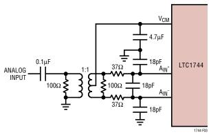
Figure 3. Single-Ended to Differential Conversion Using a Transformer
