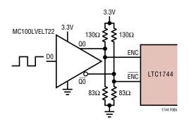
Figure 8b. ENC Drive Using a CMOS-to-PECL Translator
