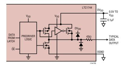
Figure 9. Equivalent Circuit for a Digital Output Buffer
