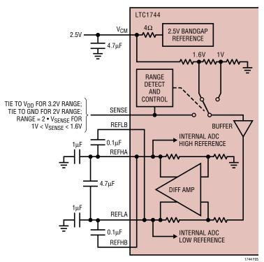
Figure 5. Equivalent Reference Circuit
