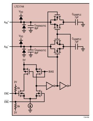
Figure 2. Equivalent Input Circuit
