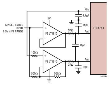
Figure 4a. Differential Drive with Op Amps
