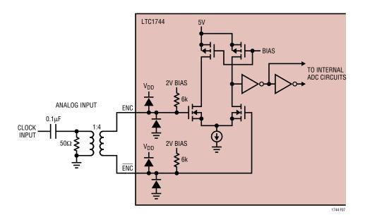
Figure 7. Transformer Driven ENC/ENC
