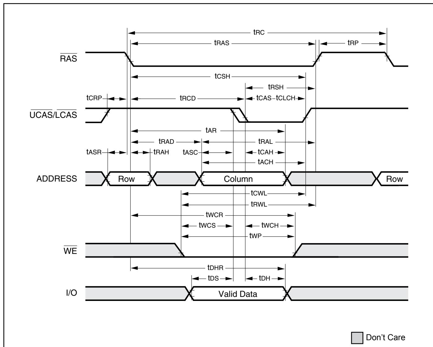
**FAST-PAGE-MODE READ WRITE CYCLE (LATE WRITE and READ-MODIFY-WRITE Cycles)**
