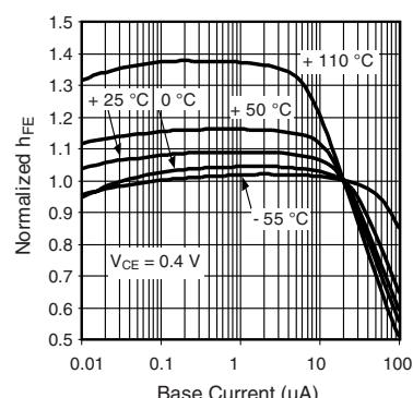
Fig. 15 - Normalized  $h_{FE}$  vs. Base Current and  $T_{amb}$
