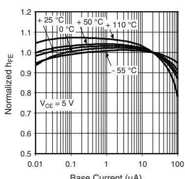
Fig. 14 - Normalized  $h_{FE}$  vs. Base Current and  $T_{amb}$
