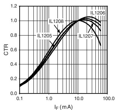
Fig. 11 - CTR vs.  $I_F$ , ( $V_{CE} = 5$  V,  $T_{amb} = 25$  °C) Normalised to
