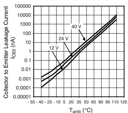
Fig. 6 - Collector to Emitter Current vs. Ambient Temperature
