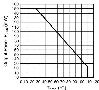
Fig. 2 - Output Power Dissipation vs. Ambient Temperature
