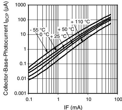
Fig. 16 - Collector Base Photocurrent vs.  $I_F$
