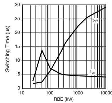
Fig. 21 - Switching Time vs. RBE,  $I_F = 10 \text{ mA}$
