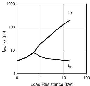
Fig. 18 - Switching Time  $t_{on}$ ,  $t_{off}$  vs. Load Resistance
