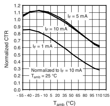
Fig. 8 - CTR Normalized to  $I_F = 10$  mA vs. Ambient Temperature,
