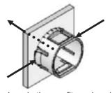
Press down both snap-fits and push the snap holder forward.
