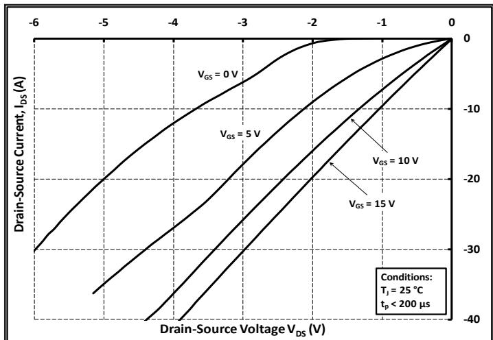
Figure 14. 3rd Quadrant Characteristic at  $25\text{ }^{\circ}\text{C}$
