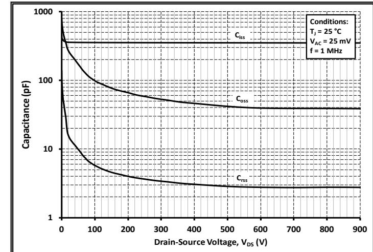
Figure 18. Capacitances vs. Drain-Source Voltage (0 - 900V)
