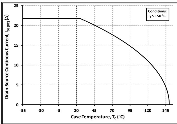
Figure 19. Continuous Drain Current Derating vs.
