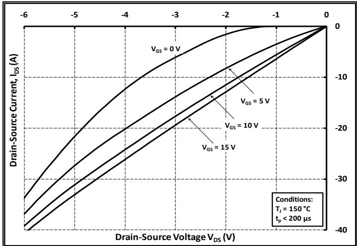
Figure 15. 3rd Quadrant Characteristic at  $150\text{ }^{\circ}\text{C}$
