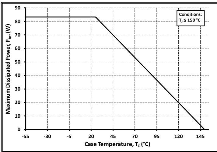
Figure 20. Maximum Power Dissipation Derating vs.
