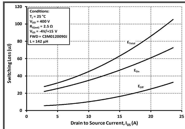
Figure 24. Clamped Inductive Switching Energy vs.
