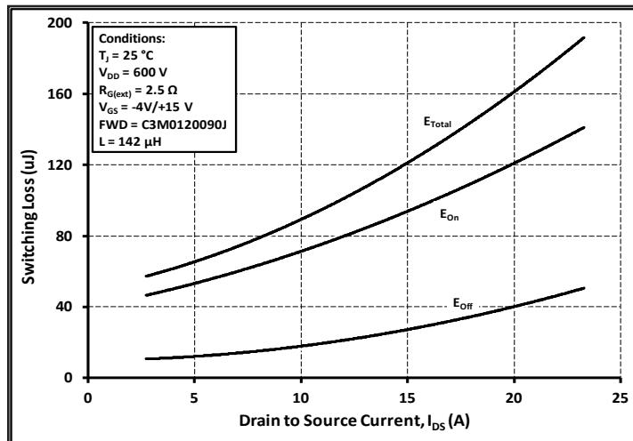
Figure 23. Clamped Inductive Switching Energy vs.
