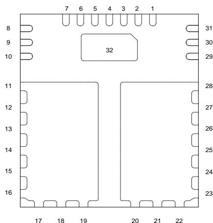
Exposed pad (Pin 32) has to be connected to COM for better electrical performance
