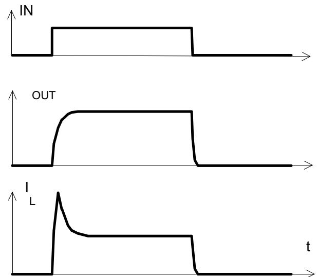
**Figure 2a:** Switching a resistive load,
