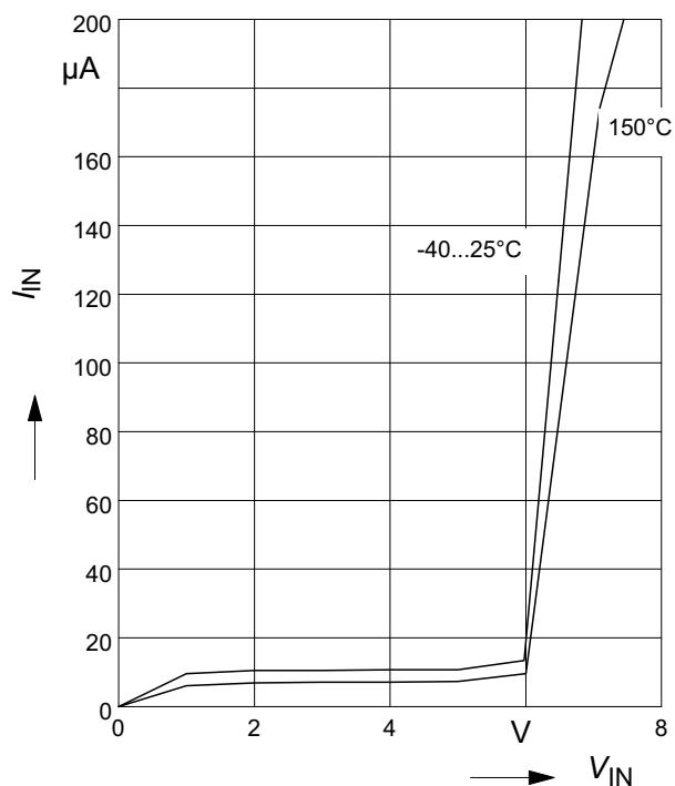
**Typ. input threshold voltage**
