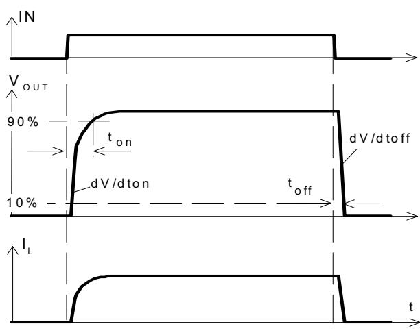
**Figure 2c:** Switching an inductive load
