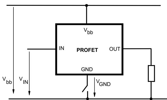
**$V_{bb}$  disconnect with charged inductive load**
