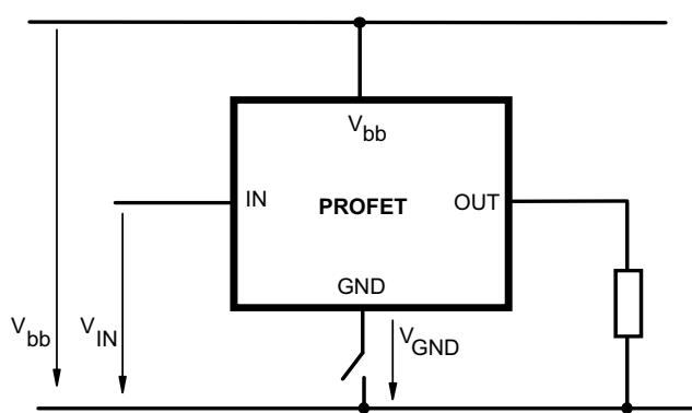
**$V_{bb}$  disconnect with charged inductive load**
