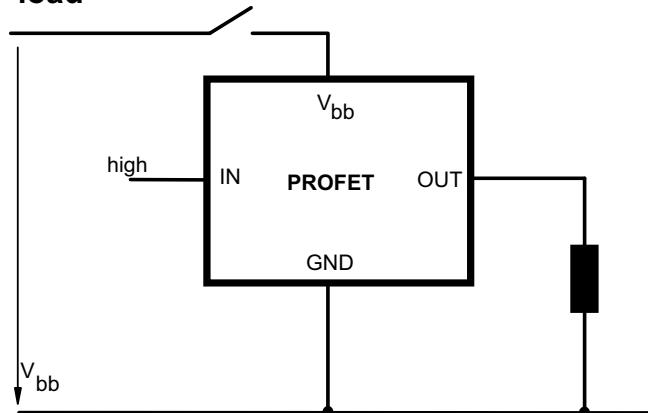
**GND disconnect with GND pull up**
