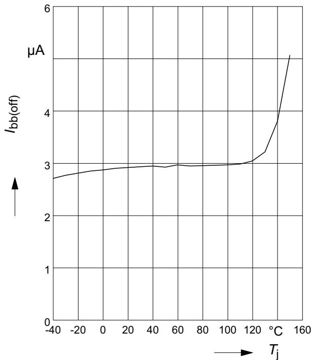
**Typ. leakage current**
