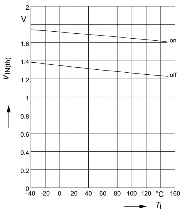
**Typ. input threshold voltage**
